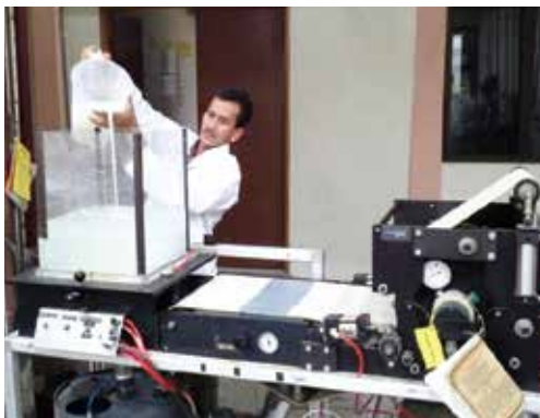
Buburan pulpa dimasukkan ke dalam tangki pada hand sheet former Pulp slurry was filled into a tank at hand sheet former
