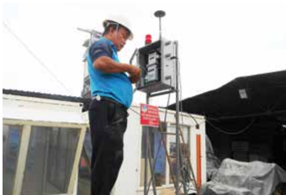
Penyediaan peralatan pemantauan habuk dan bunyi bising di kuari Preparation of dust and noise monitoring equipment at quarry
