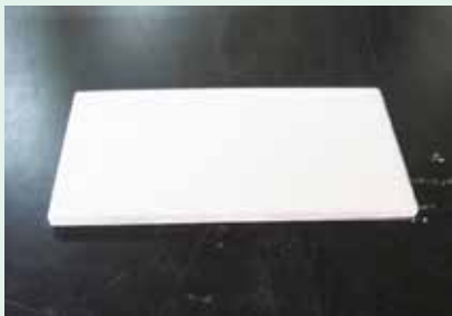
Sampel jubin kaca selepas proses pensinteran Glass tile samples after sintering
