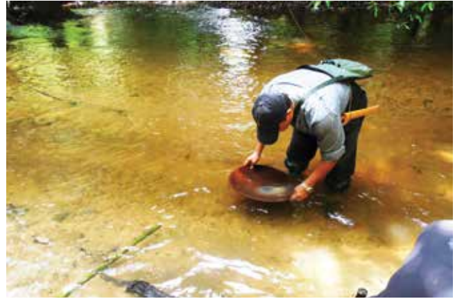
Pendulangan konsentrat mineral berat Panning of heavy mineral concentrates
