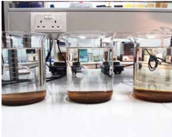
Mendakan dihasilkan melalui tindakbalas air sisa lombong dengan kapur terhidrat Precipitate produced by mixing mine water with hydrated lime
