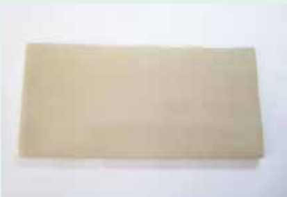
Sampel jubin kaca sebelum proses pensinteran Glass tile samples before sintering
