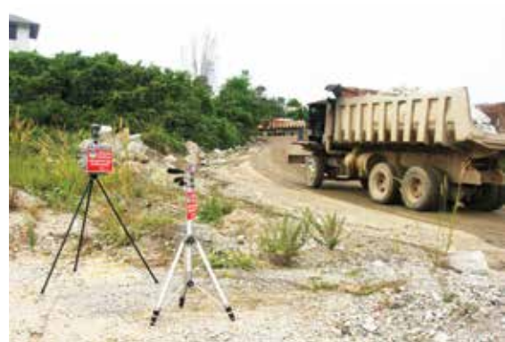
Penyediaan peralatan pemantauan habuk dan bunyi bising di kuari Preparation of dust and noise monitoring equipment at quarry
