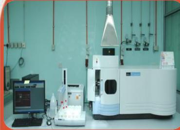
Rapid and sensitive way of measuring the elemental concentrations of solutions, up to 71 elements can be determined within detection limits of 1 part per billion
