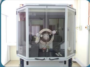
Rapid analytical technique primarily used for phase identification of a crystalline material and can provide information on unit cell dimensions
