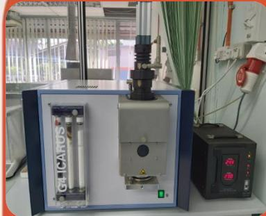
A Carbon and Sulfur Analyzer is used to analyse the percentage of carbon and sulfur present in materials
