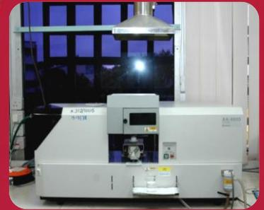
Spectro analytical procedure for the quantitative determination of Chemical elements to determine the concentration of a particular element
